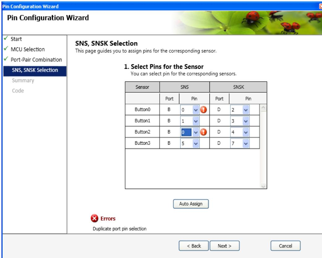
Figure 5-33: Selecting the SNS and SNSK Port Pins in the new Design( With Error)
