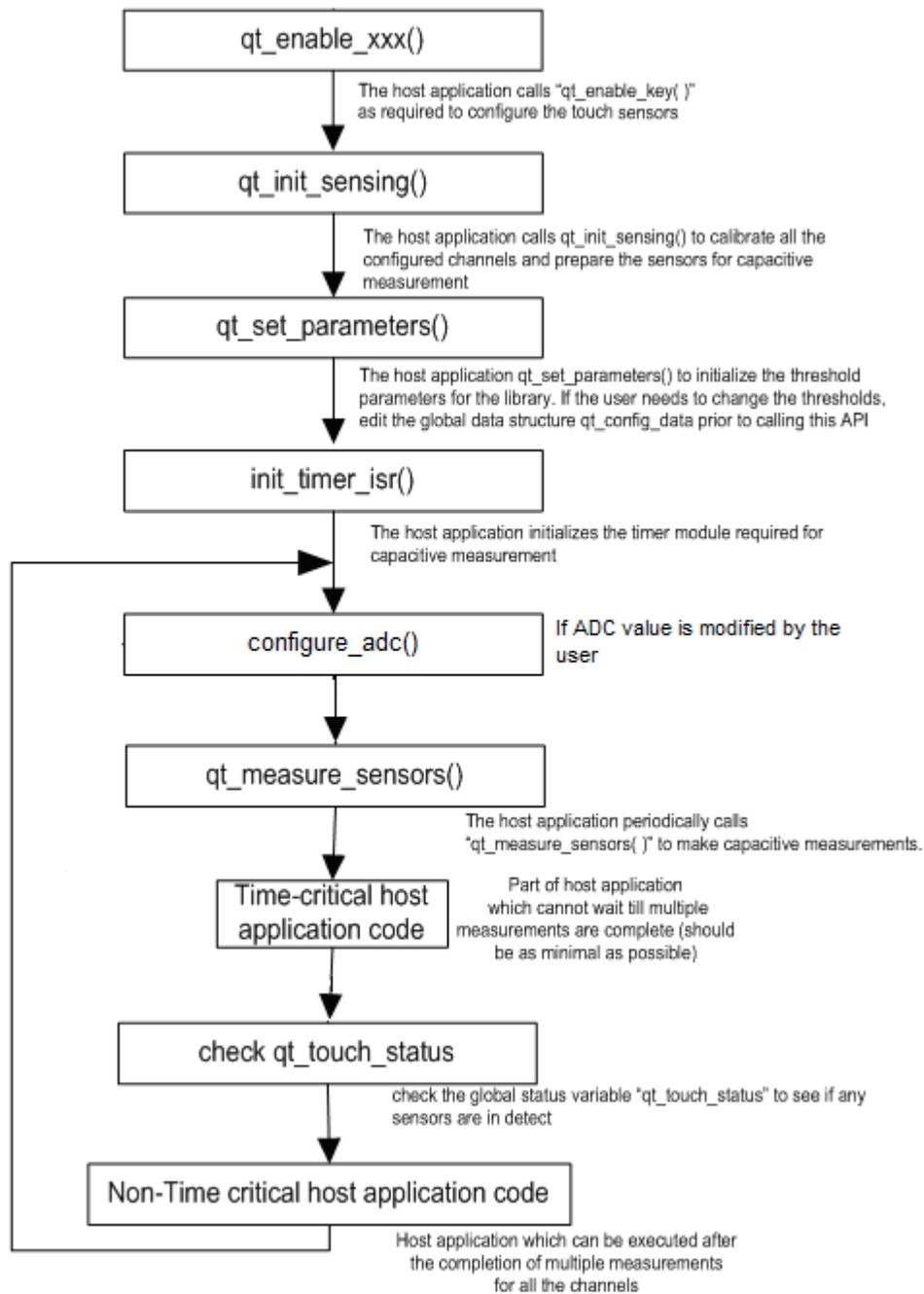
**Figure 52 QTtouch method for Tiny40 API Flow diagram**
