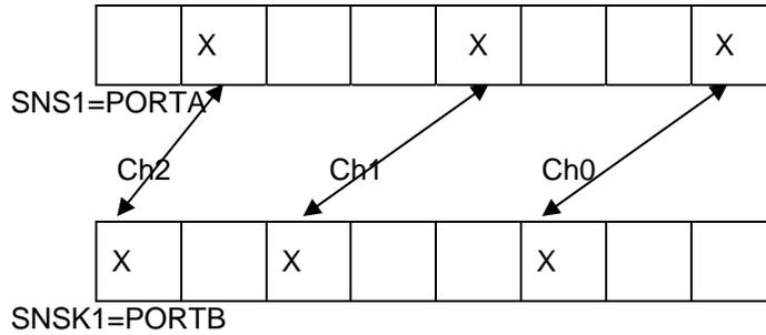
This example is for interport 8 channel library with only one port pair used. Channel0 is A0B2, Channel1 is A3B5 and Channel2 is A7B7 are enabled for the 8 channel library. The SNS\_array and SNSK\_array masks are calculated by the Qtouch Studio with rules mentioned above. In this case, the SNS\_array and SNSK\_array values will be as mentioned below:
