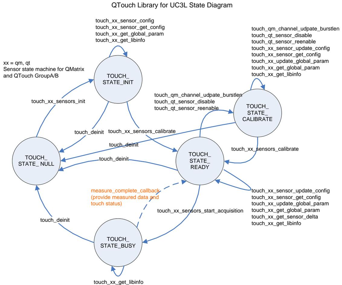
Figure 36 State Diagram of QTouch Library for UC3L
