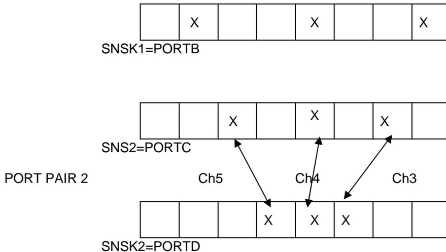
This example is for interport-interport 16 channel library with two port pair used. Channel0 is A2B0, Channel1 is A4B3 and Channel2 is A5B6 are enabled in the first port pair. Channel3 is C1D2, Channel4 is C3D3 and Channel5 is C5D4 are enabled in the second port pair.
