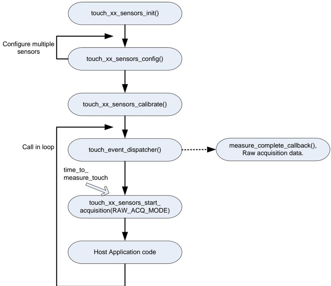
Figure 45 Raw acquisition mode API Flow diagram
