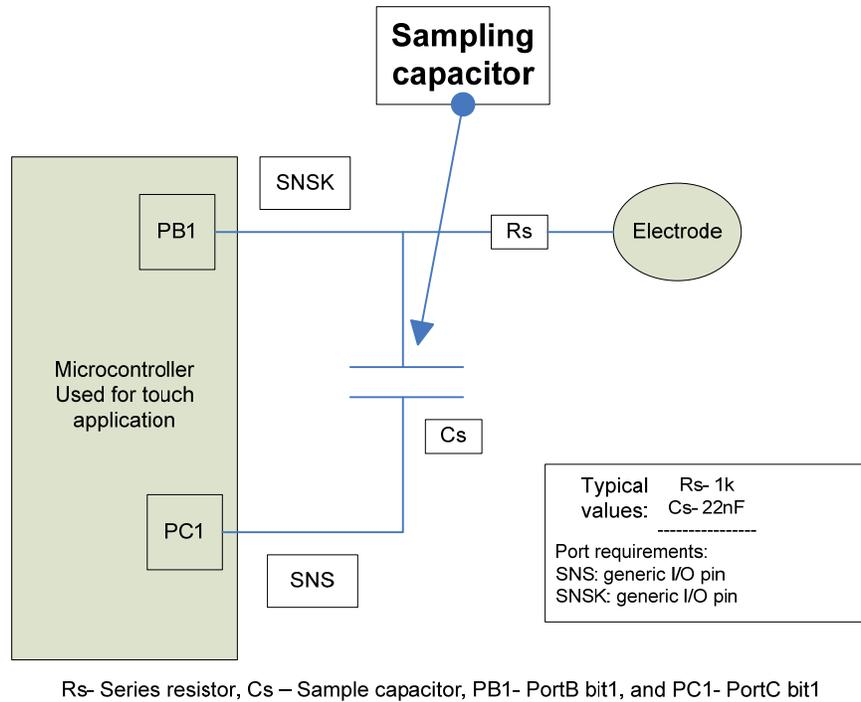
Figure 5-3 : Schematics for a QTouch acquisition method design
