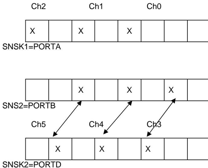
This example is for intraport-interport 12 channel library with two port pair used. Channel0 is A1A3, Channel1 is A4A5 and Channel2 is A6A7 are enabled in the first port pair. Channel3 is B1D2, Channel4 is B3D4 and Channel5 is B5D6 are enabled in the second port pair.
