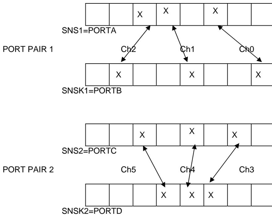
1. The channel numbers are allocated based on enabled SNS pins starting from LSBit of port 1(SNS1) and ending with MSBit of port 2(SNS2).
