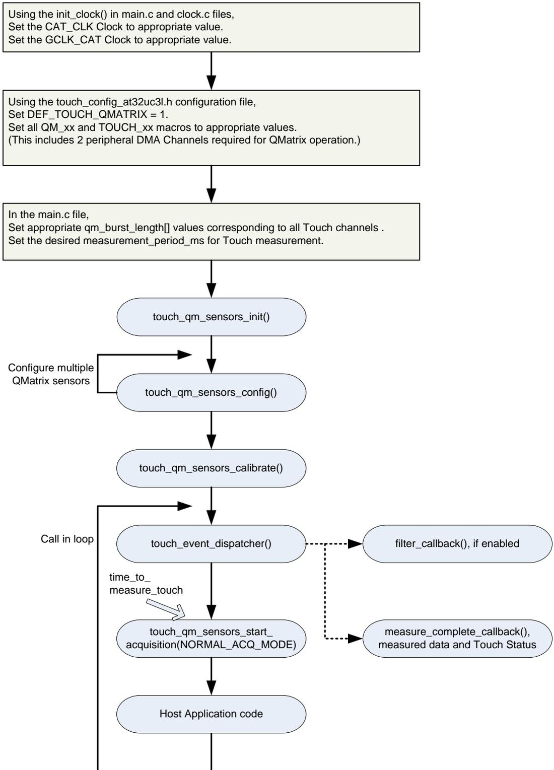
Figure 39 QMatrix API Flow diagram for UC3L
