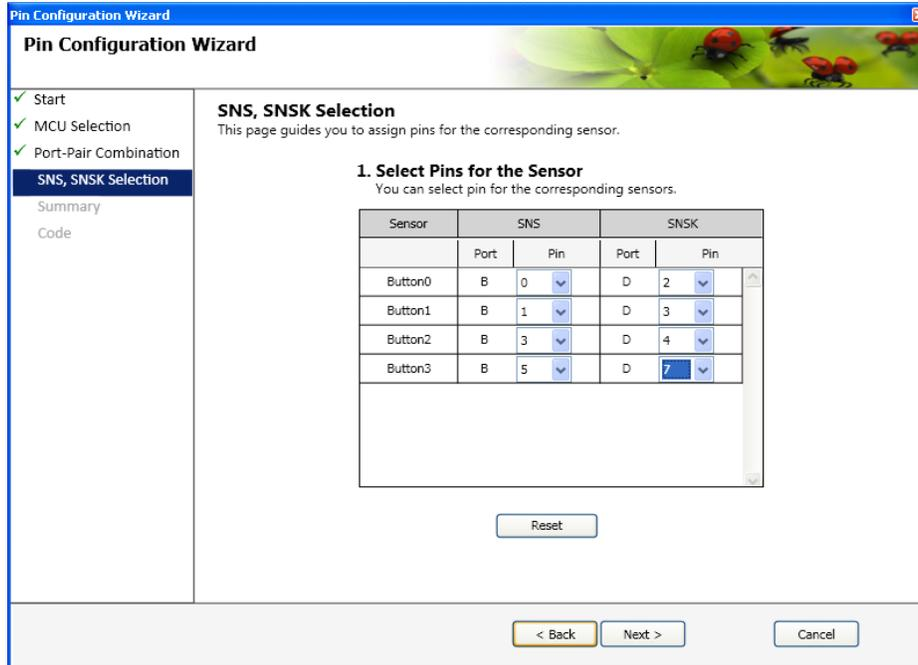
**Figure 5-34: Selecting the SNS and SNSK Port Pins in the new Design( Without Error)**
