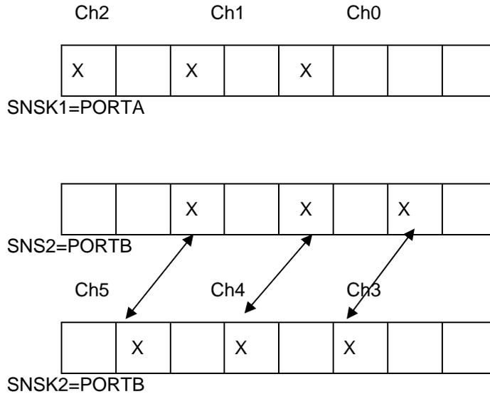
This example is for intraport 8 channel library with two port pair used. Channel0 is A1A3, Channel1 is A4A5 and Channel2 is A6A7 are enabled in the first port pair. Channel3 is B1B2, Channel4 is B3B4 and Channel5 is B5B6 are enabled in the second port pair.
