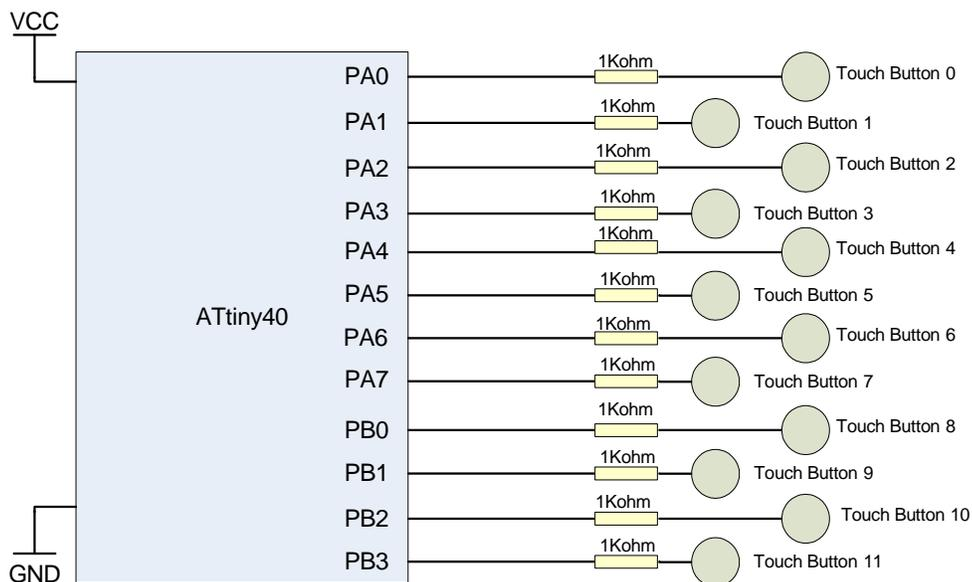
**Figure 51 Schematic overview of QTouch on Tiny40**
