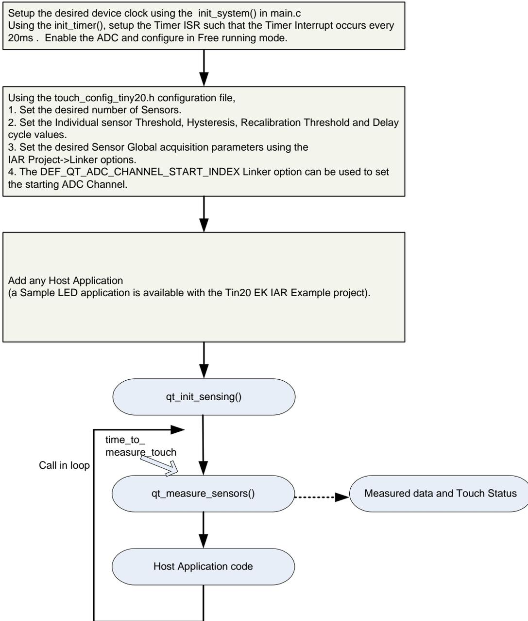
**Figure 50 QTouch method for Tiny20 API Flow diagram**
