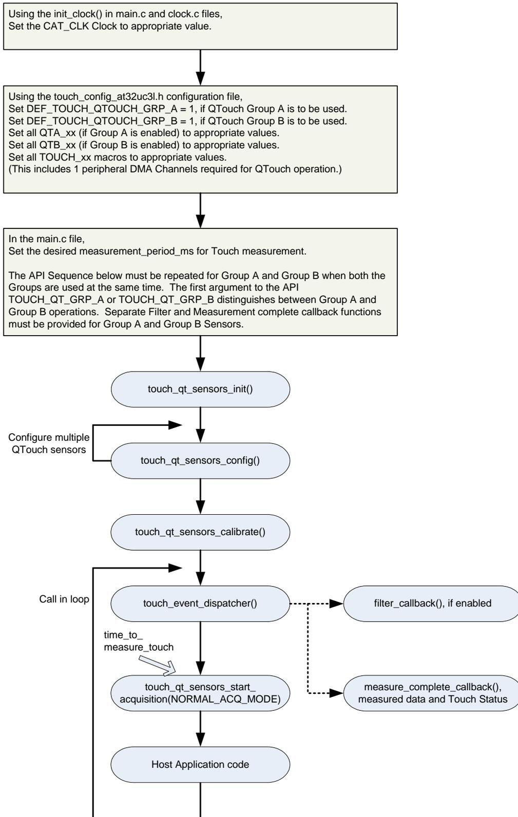
**Figure 43 QTouch method API Flow diagram**
