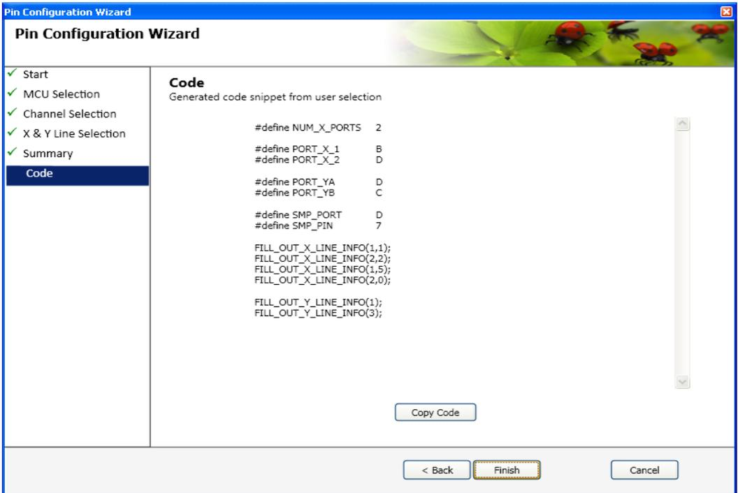
Figure 5-48: Code Generation tab in Pin Configuration wizard
